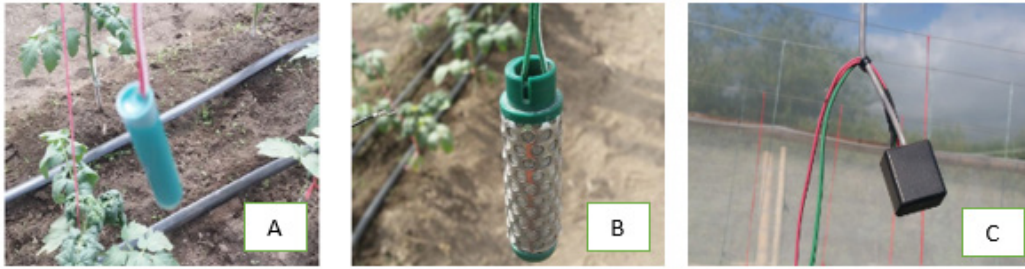
Figura 3. (A) Sensor de temperatura, (B) Sensor watermark, (C) Adaptador watermark.
